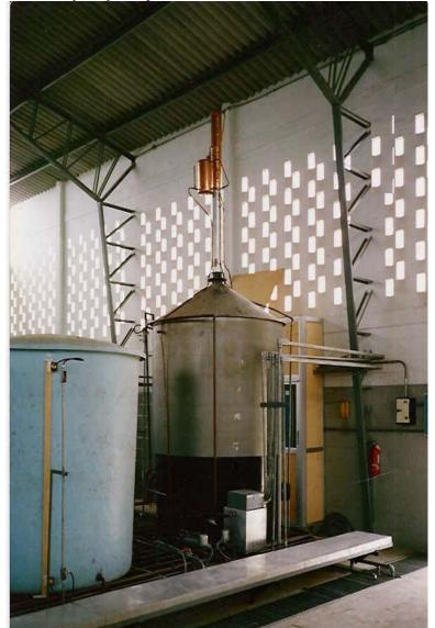
The standard model includes a temperature controlled tower, circulating water cooled condenser and insulation with aluminum jacket for added efficiency. Also standard are the brass & glass site-level and ball valves. The Still comes with two stainless steel thermometers, all instruments and a 22 pound container of distillers yeast. Column is made of copper and is completely detachable for shipment. Approx. 16'6" tall with a shipping weight of about 3,000 lbs.
