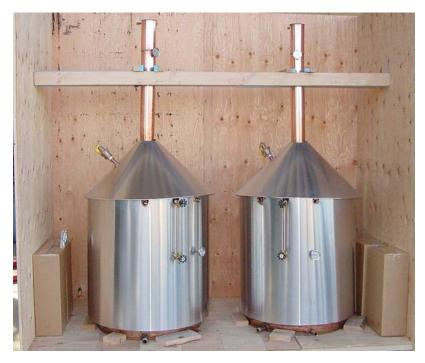
Also made of high quality heavy duty copper with brass & glass site-level and safety valve. Comes standard with insulation and aluminum projective jacket. Includes 2 stainless steel thermometers. An exceptionally productive unit! Produces about 19 to 22 gallons of alcohol in about 5 hours.
